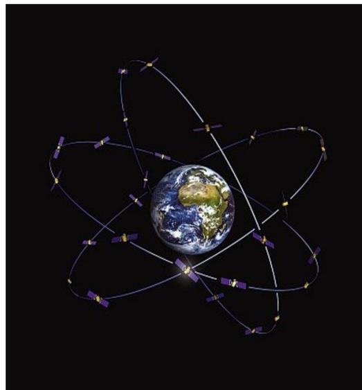
Figure 3 Galileo satellite constellation with 24 active satellites in a Walker constellation.
