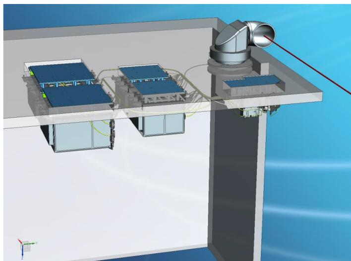
Figure 5 SMART LCT shown with the Optical Head on the right and the Communication Unit and the PAT Control electronics in a redundant scheme.
