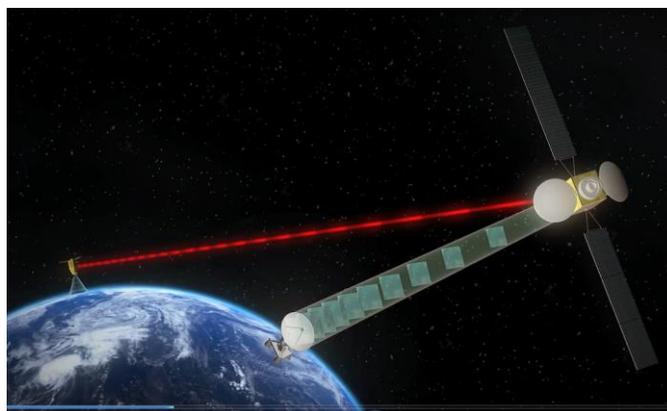
Figure 1 Data relay scheme. A LEO satellite or a UAV is sending optically a data stream (shown in red) towards the GEO satellite, shown on the right. From the GEO satellite, a Ka-Band RF transmission to a ground station follows
