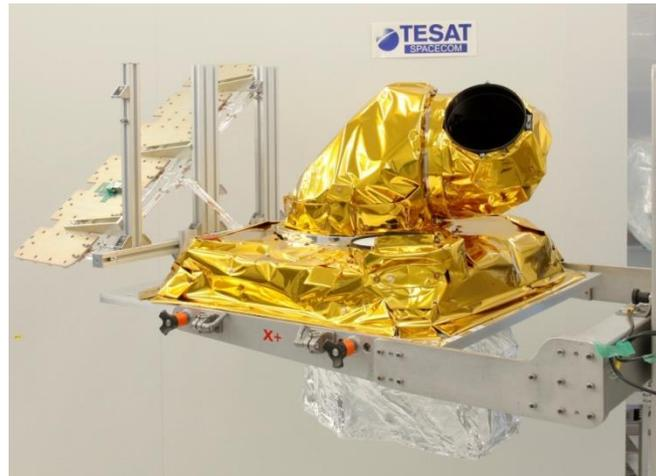
Figure 2 Alphasat LCT with Coarse Pointer opened; radiator interface is located on the left side.
