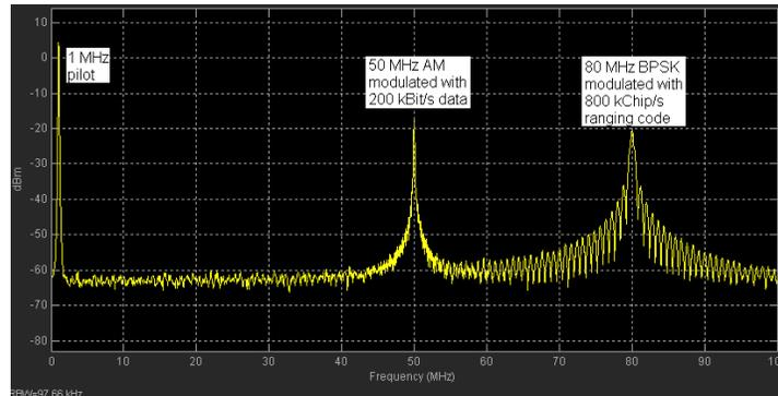
Figure 6 Transmission scheme for parallel data and ranging signal transmission.
