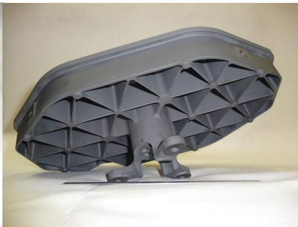
Figure 15. Ready-to-polish FoM1 FM mirror
