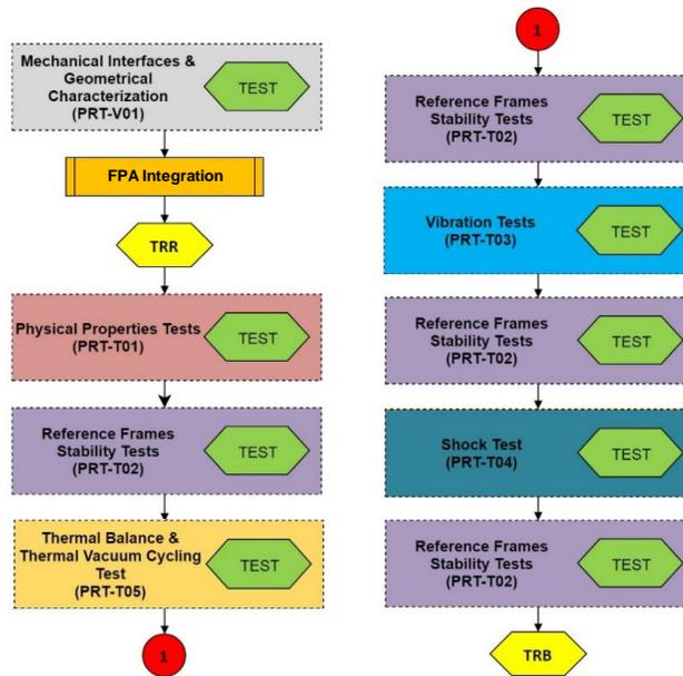
Figure 8: PRT Test Campaign Sequence
