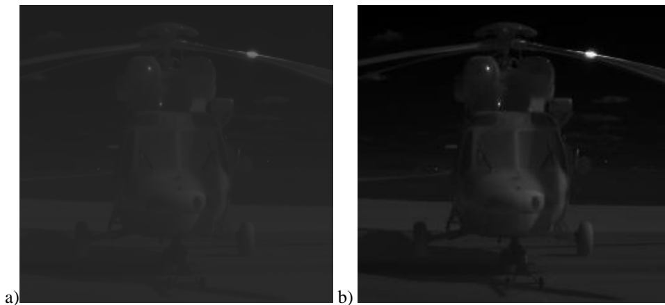
Figure 3. Example of applying LUT operation for image normalization: original image (a) image after normalization (b).
