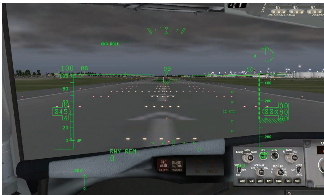
Figure three: X plane display with HUD Symbols on initialisation
