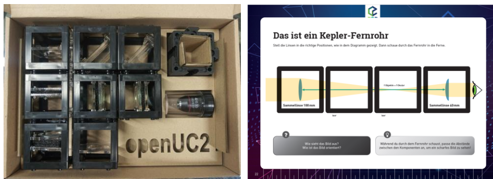
Fig. 1. Left: openUC2 MiniBOX prototype (injection moulding/ laser cutting); Right: Example from the MiniBOX booklet – manual to build a Keplerian telescope.
