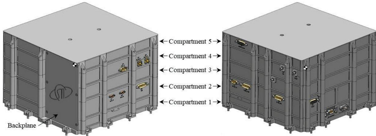
Figure 1. CAD of the EM Laser Head.
