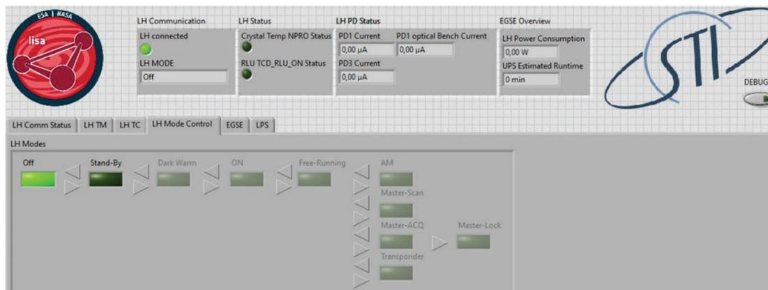
Figure 4. LabVIEW user interface to toggle between different operational modes of the LH. Bright green shows the current operational mode.
