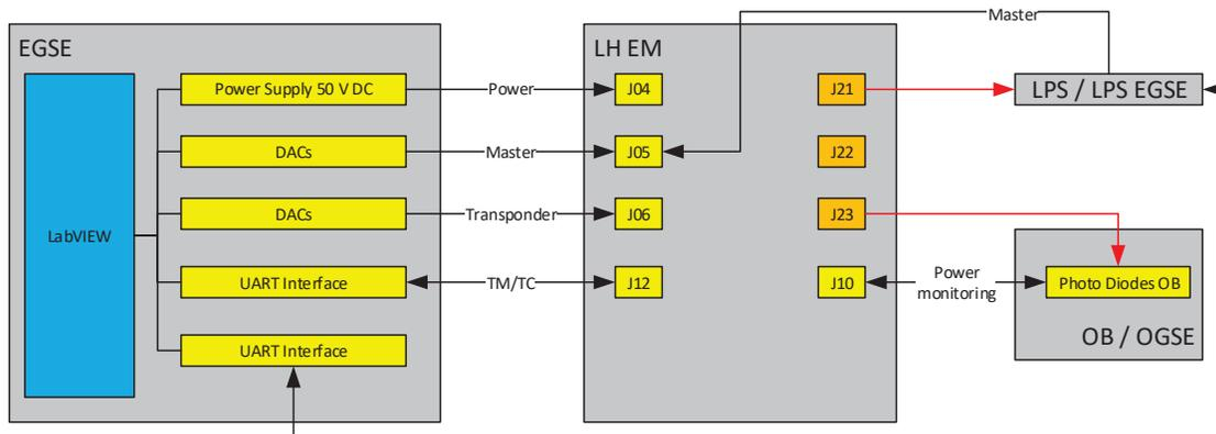
Figure 3. Overview of the setup to operate the EM LH.
