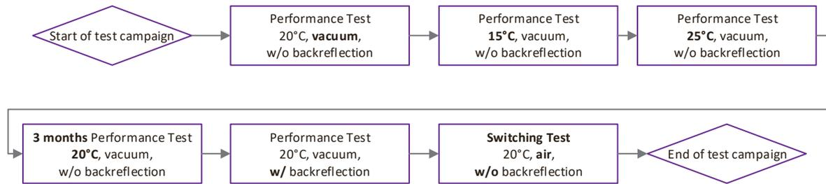
Figure 6. Flow diagram of the LH test campaign.
