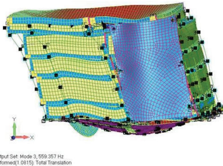
Figure 2. First main mode in x at 559 Hz (in-plane).
