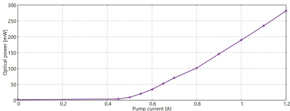
Figure 5. Optical power at the output of the first amplifier stage.
