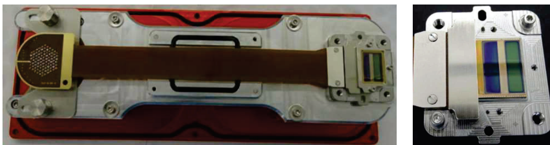
Figure 12 : Lynred EM Detector for TRISHNA TIR instrument
