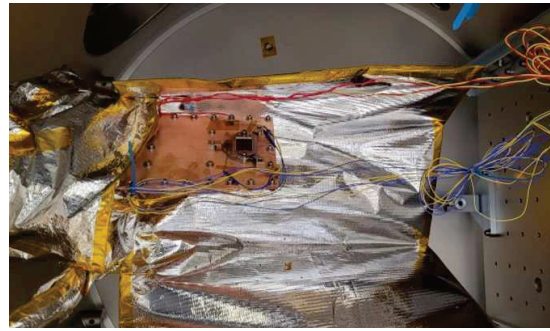
Filters support BB thermal cycling under vacuum
