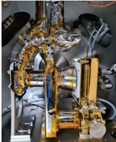
Cold-vacuum optical setup with DM Lynred detector
