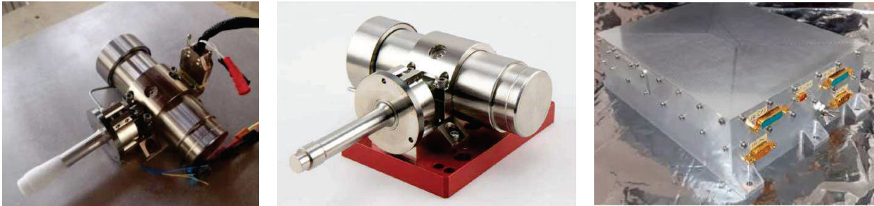
CMA EM2 during magnetic moment test
