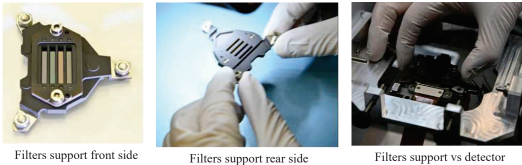
Figure 7 : Filters mounting on detector package
