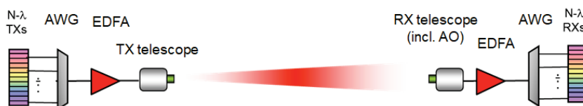
Figure 2: Structure of the WDM FSOC system, including (de-)multiplexers, amplifiers (EDFA) and telescopes.
