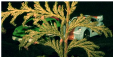
Fig. 4. 3D object used in the experiments. The blue car is a true class target, green car is a false object. Vegetation is positioned in front of the cars to partially occlude the background objects.
