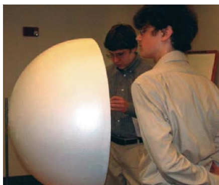
Figure 4. High school students experiment with a home-made Styrofoam integrating sphere.
