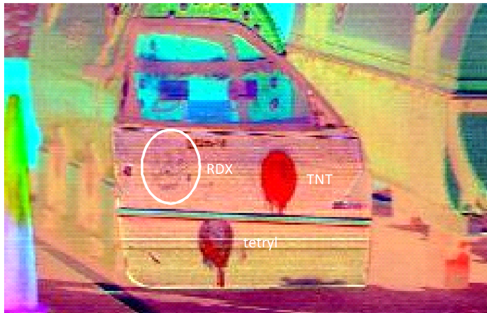
Figure 4. Shown above is a color mapping of PC components 6, 7, and 8 into the red, green and blue display colors, respectively. Note that the outline of the RDX residue patch is also visible in the image that is not apparent in a normal intensity image.
