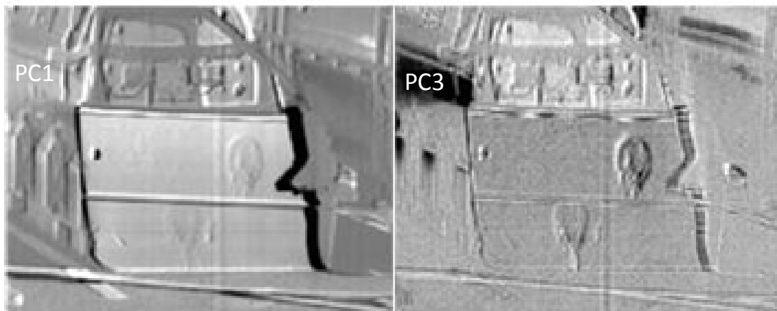
Figure 5. PC components 1 and 3 are shown that reveal the scattering from the TNT (upper) and tetryl (lower) stains on the car door. The RDX residue was not evident in any of the Q image components or subsequent principal component transform.
