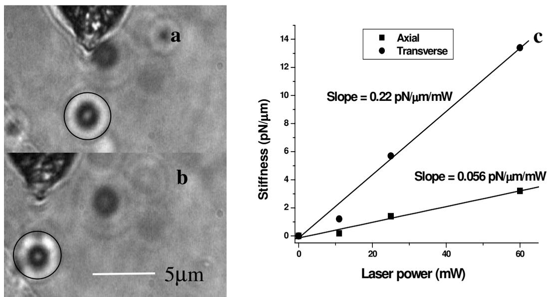
**Fig. 2** (a) Image of a trapped 2- $\mu\text{m}$  polystyrene particle (circled). (b) Transportation of the trapped particle by maneuvering the fiber tip. (c) Plot of measured stiffness along axial and transverse directions for the 2- $\mu\text{m}$  particle as a function of trap beam power.
