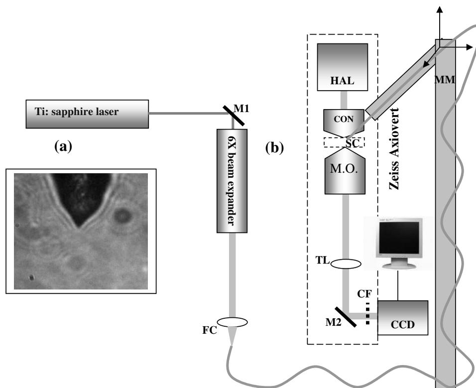
**Fig. 1** (a) Microscopic image of the tapered tip with 60-deg cone angle. (b) Single-fiber optical tweezers and scissors setup. M1, M2: folding mirrors; M.O.: microscope objective; SC: sample chamber; CON: condenser; HAL: halogen lamp; FC: fiber coupler; MM: motorized manipulator; CF: IR cutoff filter; TL: tube lens.
