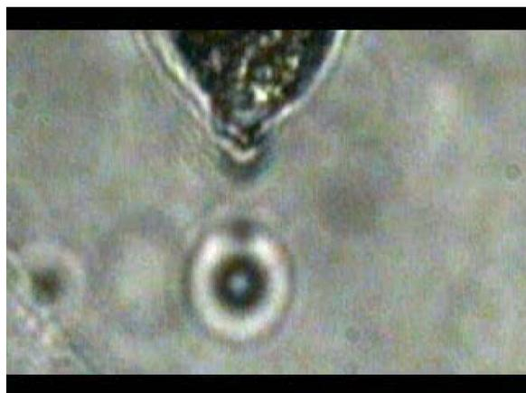
**Video 1** Video showing 3-D trapping of a 2- $\mu\text{m}$  polystyrene particle using a 90-deg cone angle fiber tip. Transportation of the particle can be achieved by translation of the fiber. Video corresponds to data in Figs. 2(a) and 2(b). Resolution is  $320 \times 240$  (MPEG,  $\sim 2$  MB). [URL: <http://dx.doi.org/10.1117/1.2983663.1>].
