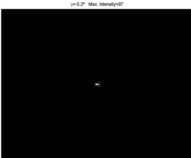
Video 1 Retinal PSF at different incidence angles. Each frame has been normalized to its maximum value. Notice that the best image is obtained at \gamma = \pm 5.2 deg (MPG, 5.4 MG). [URL: http://dx.doi.org/10.1117/1.3158996.1 ]
