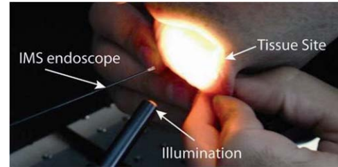
Fig. 13 Experimental setup for imaging the tissue vascularization of the lower lip of a normal volunteer.
