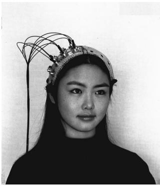
Fig. 4 The optical topography interface (a 12-channel instrument).
