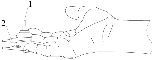
Fig. 1 Schematic presentation of the LDF probe positioning on a finger: (1) LDF probe and (2) pulseoximetry sensor.
