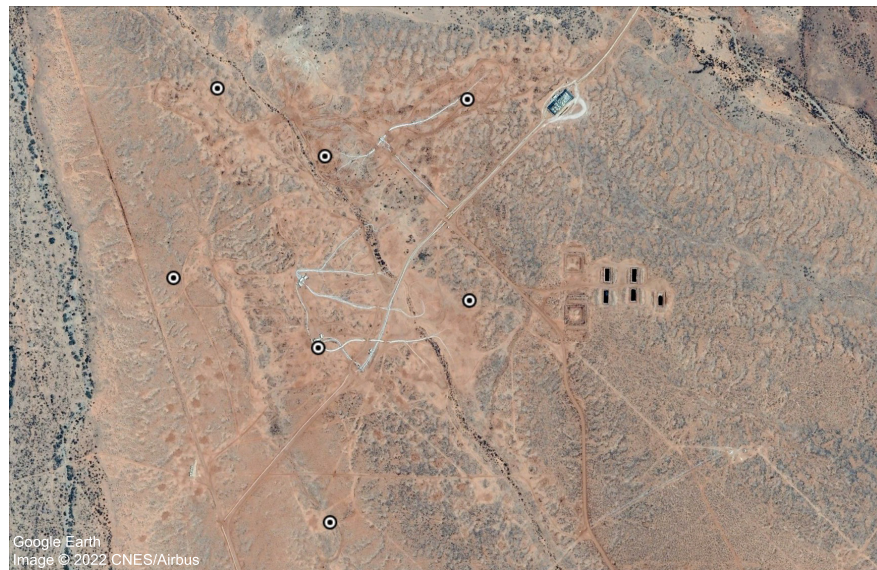
Fig. 2 Overhead image of Four Mile mine, East section, with locations of monitoring wells marked with black and white targets; 7 image is from Google Earth (CNES/Airbus, 2022). Spatial coverage is the same as that for the InSAR analysis.
