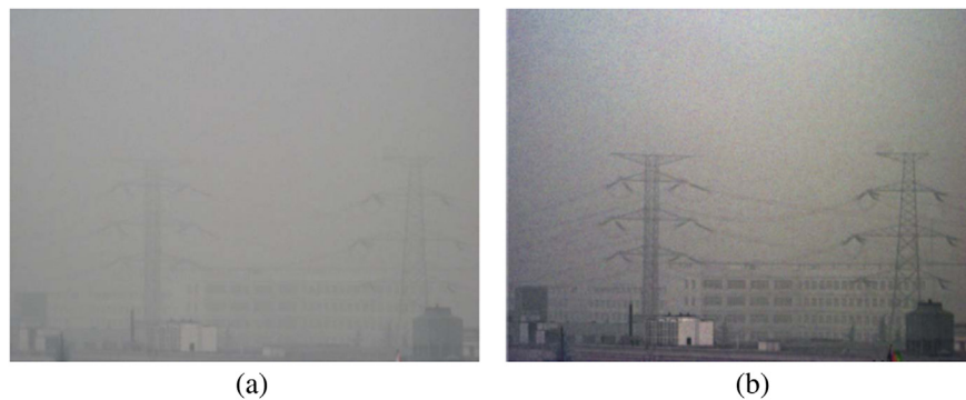
Fig. 18 (a) Fused image of visible and near-infrared hazy image. (b) Fused image of visible and near-infrared dehazed image, i.e., the final dehazing result. 88
