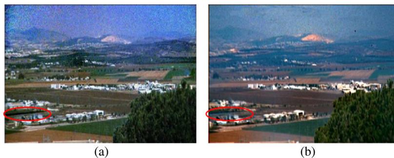
Fig. 9 (a) Dehazing results using Schechner's method in Ref. 42. (b) Dehazing result with consideration of the polarization effect of the objects using the proposed method in Ref. 57.
