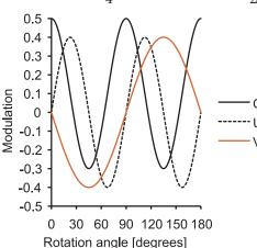
A waveplate with  $\delta=126.8$  deg at the wavelength of interest has equal modulation amplitudes and sensitivity for Q, U, and V. The rotation can be continuous with eight equally long integrations per rotation or stepped to four or more discrete angles.
