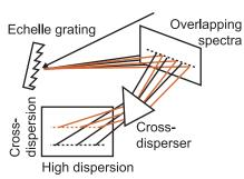
Overlapping Spectra becomes too small. However, the spectral overlap can be avoided by spatially separating the diffraction orders by means of a so-called pre-disperser, a low-dispersion prism or grating. Since the pre-
