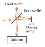
A Fourier transform spectrometer (FTS) is a classical Michelson interferometer with a variable path length L and detectors and beamsplitters appropriate for the considered spectral range. The change in path length occurs with constant velocity or by stepping, the latter enabling imaging FTS instruments.
