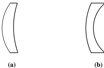
Figure 2-19. (a) Positive and (b) negative meniscus lens. The radii of curvature of their surfaces have the same sign. The lens thickness at the center is higher compared to that at the edges for a positive meniscus, and lower for a negative meniscus.
