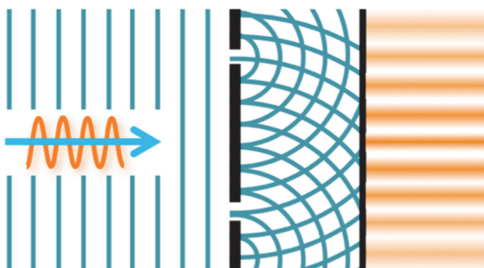
Figure 1 When light, in the form of a plane electromagnetic wave, passes through two slits in a screen, it diffracts and creates bright and dark fringes on a detector screen (screen and pattern shown on the right-hand side). The effect is commonly explained in terms of constructive and destructive interference of the diffracted wave at different positions.
