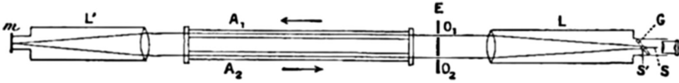
Figure 1.4 Reciprocal ring interferometer used by Fizeau to demonstrate the matter drag effect in 1851: a source S is placed at the focal point of a lens, and the collimated beam goes through two holes ( O_1 and O_2 ) to yield two parallel beams that propagate in the moving water and that are swapped on a cat's eye (on the left) to return “reciprocally.”
